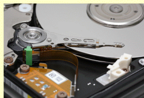
Modern hard disks make use of GMR. (Image credit: http://commons.wikimedia.org/wiki/User:Mfield , Creative Commons Attribution ShareAlike 3.0)
