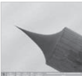
Figure 3: SEM image of a tungsten tip for STM imaging
