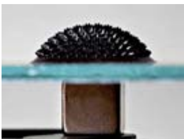
Figure 9: Ferrofluid with a magnet underneath
