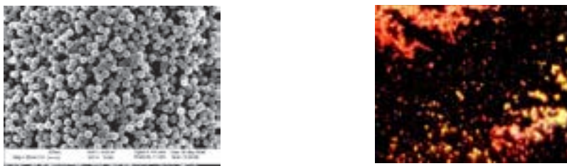
Figure 7: (left) SEM image of gold nanoshells each being about 120 nm; (right) optical image of the same nanoshells after being dispersed in water and dried on a microscope slide. The colours are due to selective scattering of light by the nanoparticles.
