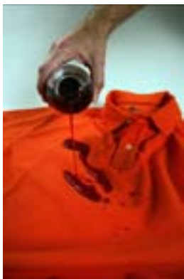
Figure 7: Liquid staining on a Nano-Tex® fabric
