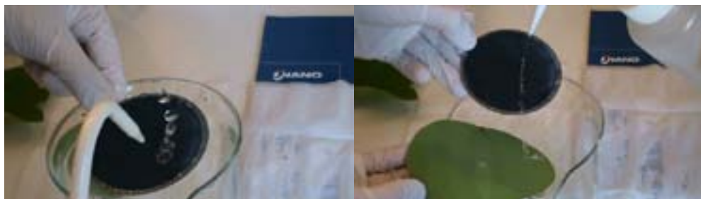
Figure 9: Images from NANOYOU Video 4 — Lotus effect ® , Part 2 — showing the wetting properties of a piece of porous silicon (left) and how this material compares with a real lotus leaf (right)
