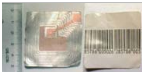
Figure 8: RFID chip on a stick with barcode on the opposite site
