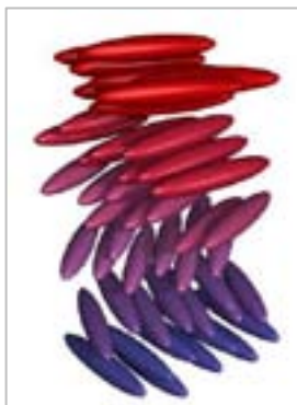
Figure 5: Schematic representation of ordering in chiral liquid crystal phases: a chiral nematic phase (also called the cholesteric phase) in a liquid crystal
