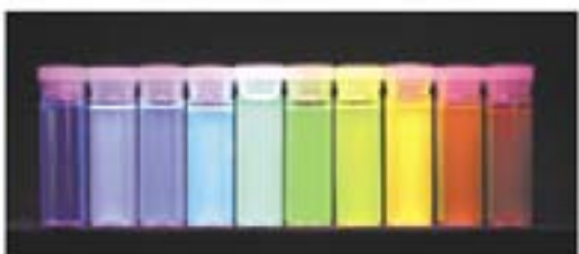
Figure 11: Ten distinguishable emission colours of ZnS-capped CdSe QDs excited with a near-UV lamp
