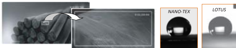
Figure 8: (left) High resolution images of the Nano-Tex® fabric; (right) contact angle images of water droplets on Nano-Tex® fabric and lotus leaf
