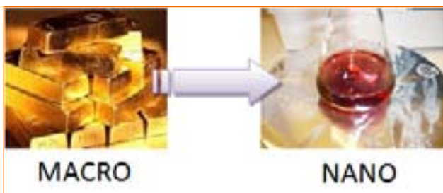
Figure 4: Dependence of colour on gold size
