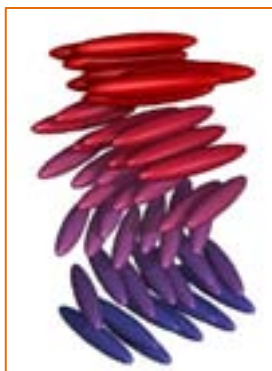
Figure 3: Schematic representation of ordering in chiral liquid crystal phases: a chiral nematic phase (also called the cholesteric phase) in a liquid crystal
