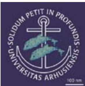
Figure 14: Researchers began by cutting a dolphin out of the University of Aarhus logo, which was then used as a template to design a dolphin-like DNA structure. After producing this in the laboratory, AFM images were taken of the DNA structure thus formed and an image of the DNA dolphin was reinserted in the Aarhus University logo.
