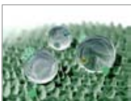
Figure 6: Diagram summarising the connection between roughening and self-cleaning: (top) a droplet of water removes dirt from a surface due to the Lotus effect®; (bottom) graphical representation of contaminants and water droplets on a lotus leaf
