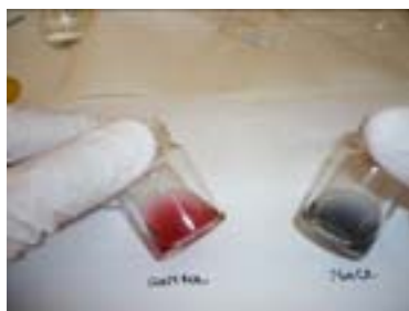
Figure 11: Colour change as salt is added to the gold colloid
