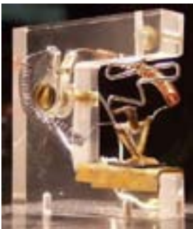
Figure 1: Replica of the first bipolar transistor, this replica was photographed at the Nixdorf-Museum, Paderborn, Germany.
