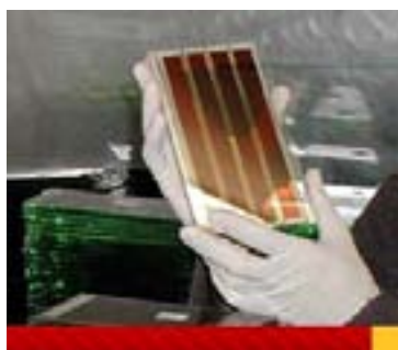
Figure 4: A dye solar cell (DSC) commercialised by DyeSol
