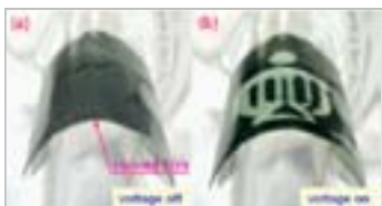
Figure 7: Thermochromic display under development at the Hong Kong University of Science and Technology
