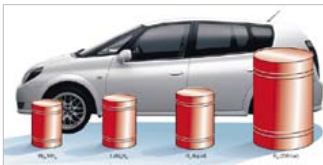
Figure 7: Volume of 4 kg hydrogen compacted in different ways, relative to the size of a car
